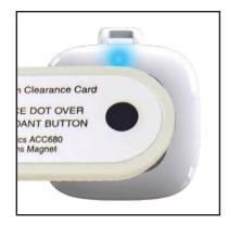
A Series of Six Blue Flashing lights will indicate a successful alarm clearance.
