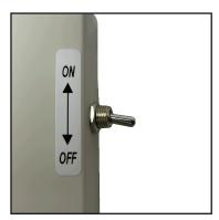
**Turn Off**Begin with the transmitter switch in the off position.
