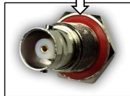
**3.** From the inside of the case insert the BNC connector through the hole, place the flat washer, lockwasher, and secure with the 1/2" nut.
