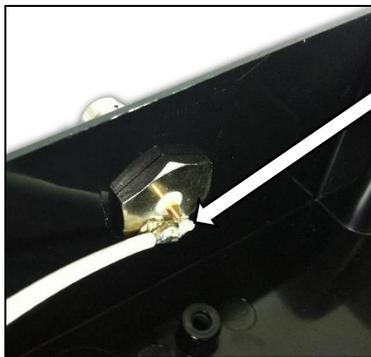
**4a. BNC installed in the case top**
