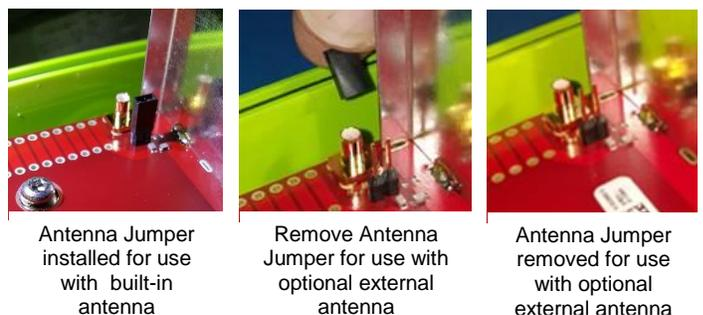
Antenna Jumper installed for use with built-in antenna      Remove Antenna Jumper for use with optional external antenna      Antenna Jumper removed for use with optional external antenna
