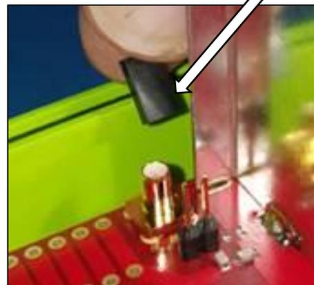
**7.** With the external antenna connected to the BNC connector, tightly wrap the entire connection with the black silicon tape included in the 60201125 antenna connector kit.
