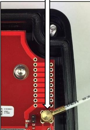
**6. REMOVE** the Antenna Jumper for use with an optional external antenna.
