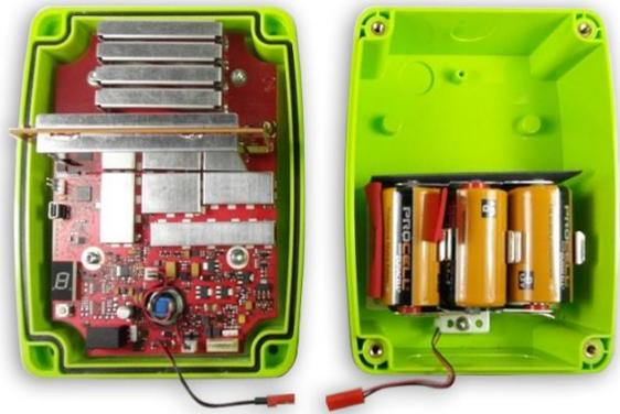
**Using External +12 VDC Power with Battery Back-up**
