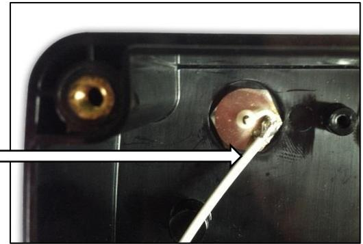
**4c.** Once positioned, tighten the 1/2" nut while holding the BNC connector in place with a 1/2" open end wrench. Be sure the nut is completely tightened to form a good weather seal with the sealing washer.
