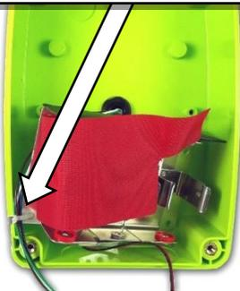
⑧ Tighten the Tie Wrap after the battery holder is installed. Connect the 6-Conductor cable to the RQX XD-Series radio.
