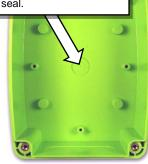
Install the Heyco strain relief as shown. Thread the 6-conductor cable through from the inside.
