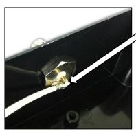
**4a.** BNC installed in the case top Position the connector so that the cable is routed as shown, downward toward the inside of the case back.
