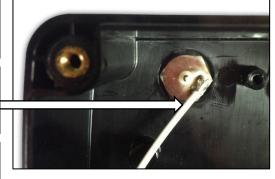
7. With the external antenna connected to the BNC connector, tightly wrap the entire connection with the black silicon tape included in the 60201125 antenna connector kit.
