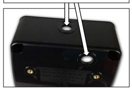
2. Before installing the BNC connector into the case, place the sealing washer on the connector as shown. Be sure it is completely seated in the recessed area and is flat, with no twist or binding.
