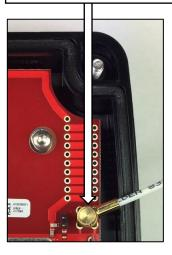
**6. REMOVE** the Antenna Jumper for use with an optional external antenna.
