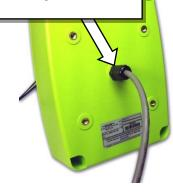
Pull the 6-conductor through as shown until there is less than ¼ inch of the gray sleeve showing through the strain relief. Use the Inside Retaining Nut to tighten to case, then tighten the Cable Sealing Nut.
