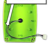
Use the Cable Tie to secure the 6-conductor cables to the battery holder as shown. The 6-conductor cables will run beneath the battery holder. <u>Do not tighten the Cable Tie at this time.</u>
