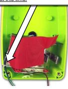
WARNING! Be sure the wires are not trapped between the battery holder and the molded plastic mounting stud! Wires are routed below the stud as shown.
