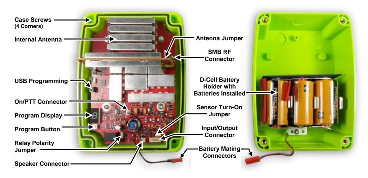
FIG-2: Callbox Assembly, Controls and Connectors
