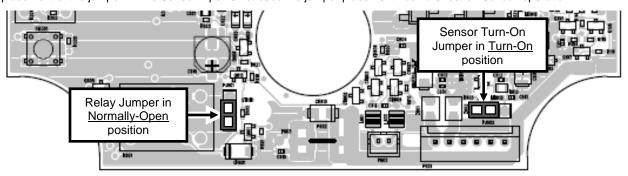
FIG-1: Sensor Turn-On Jumper Shown in Turn-On Position
