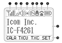
**1** SIGNAL STRENGTH ICON Displays the relative receive signal strength.
