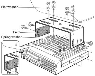
When using self-tapping screws
